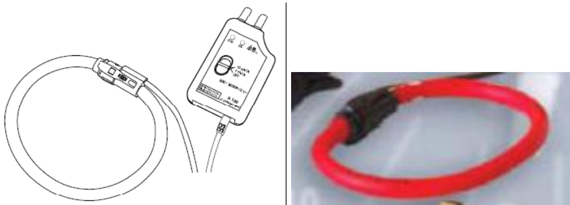
Figure 2-12. Flexible Rogowski Coil with Integrator
