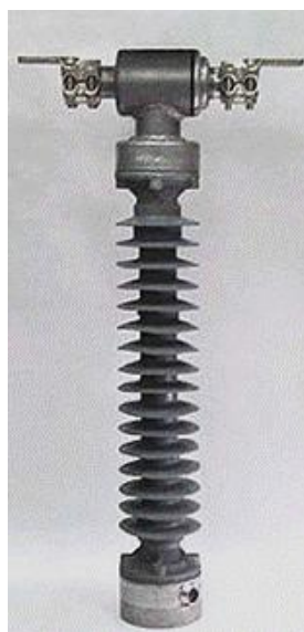
Figure 4-14. Stand-Alone Rogowski Coil for Current Measurements at 69 kV, 1200 A (44 lb)
