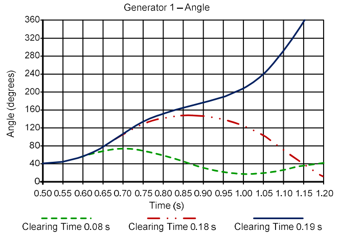
Fig. 19. Angle Versus Time for Generator 1 for Bolted Three-Phase Faults at Line L_4-5 from Node 4
