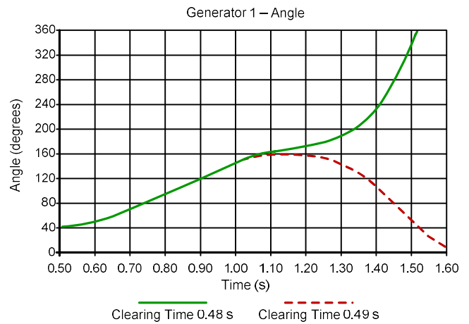
Fig. 20. Angle Versus Time for the Generator 1 for Three-Phase Fault at 20 Percent Over Line L_4-5 at Node 4
